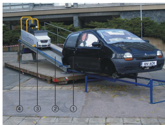
Figure 2. The crash simulator at a safe distance nonobservance prototype [author].
